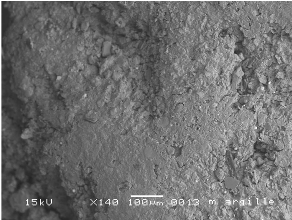
Fig. 4.30 Merville clay sample with a shear band: smooth surface.
